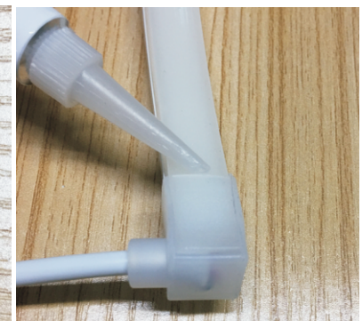
Step 10: Put more silicon glue around the wire and all the side. Step 11: do not move it , and Waiting until Glue is dry fully in 2-3hours.
