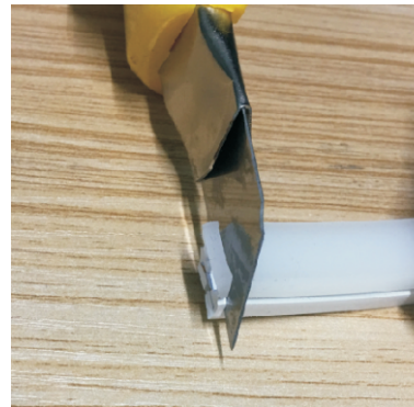
Step 3: Cut off the silicon to get the Soldering Point of the FPC.
