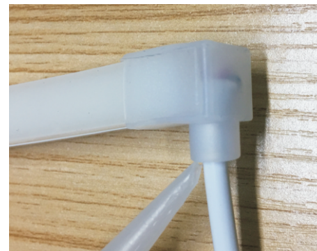
Step 10: Put more silicon glue around the wire and all the side. Step 11: do not move it , and Waiting until Glue is dry fully in 2-3hours.
