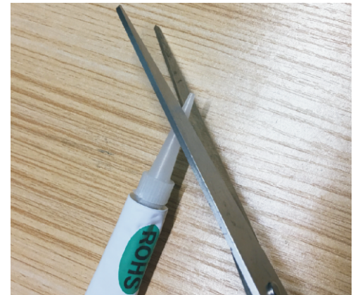
Step 7: Cut off the mouth a little for Glue passing.
